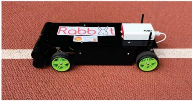
FIG. 1. The line following robot. It is built of an RC car, with the Raspberry Pi under the top plate. A 5V battery is on top of the car, and directly connects to, and powers the Raspberry Pi. The ultrasonic sensors are attached on the front of the bumpers, and the IR sensors are under the bumpers.
