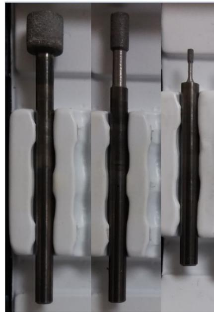
FIG. 3. Left to Right: 6.35 mm, 3.175 mm, and 1 mm Bits
