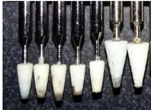
FIG. 5. Felt Bobs for Polishing
