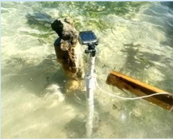
Figure 9. Experiment 4: Rock depth. Outdoor experimental setup to assess the tidal threshold that periwinkles can withstand. A 60cm long coral rock was placed with 11cm exposed ( n=10 ). A time-lapse camera attached to a pole driven into the sea sediments recorded periwinkle movements.
